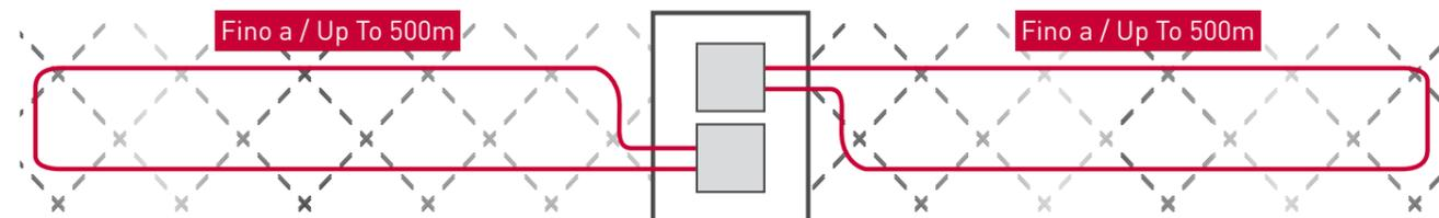
**CONFIGURAZIONE A CATENA PER RECINZIONI ALTE FINO A 2,5M / DAISY CHAIN CONFIGURATION UP TO 2,5M HIGH FENCES**
