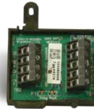
The FC410MIM Mini Input module is designed to monitor fire contacts, such as extinguishing system control, ventilation control, fire door control etc. The module provides one identifiable detection spur which is capable of monitoring multiple normally open contacts or a single normally closed contact.
