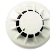
The 702H and 703H heat detectors detect abnormally high static temperatures of 60°C and 90°C, respectively. They can be used in areas where smoke detectors are unsuitable due to environmental conditions such as kitchens, locker rooms and canteens.
