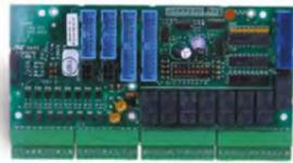
The IOB800 input/output expansion module is an LPCB approved board that provides 8 opto isolated digital inputs and 8 x 24Vdc relay outputs for providing I/O expansion capabilities to the FireClass control panels for interfacing to other fire protection systems and signalling devices. The IOB800 can be driven from either the control panel or from the remote bus.
