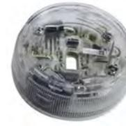
The FC442AVB is an addressable open class VAD sounder beacon specifically for use with FireClass addressable detectors. The base incorporates a fire alarm sounder, carrying its own address which can be monitored and controlled from the fire alarm control panel independently of the detector. Both power and communications for the sounder and detector are provided by the FireClass digital loop.
