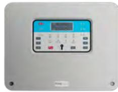
FireClass Essential Panels are EN-approved, low cost conventional panels that are available in both 2 Zone and 4 Zone variants. The panels can support up to 128 devices with a maximum of 32 devices on each zone. The panels are approved to EN 54-2, EN 54-4, and listed as part of the EN 54-13 system certificate.
