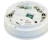
Functional detector bases use a common moulding which incorporates a double sided circuit board which enables electrical connections to be made on the top and bottom of the functional base. This allows the functional bases to be retrofitted into new and existing universal bases or alternatively the depth and cost of the installed detector can be reduced by using the functional base instead of the universal base.
