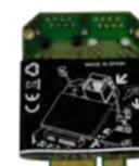
The ONE500-Loop is an expansion card that allows users to connect up to 10x ONE500 with a total of 60 zones. The expansion card ONE500-LOOP has a redundant communication which allows the systems to be supervised and managed according to EN54 standards.
