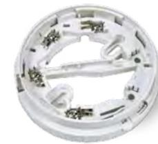
The 4B-I 4" Isolator base is designed to snap-fit to the ceiling tile adaptor or it can screw fix to a ceiling in the traditional manner. The 4B-I 4" base is designed specifically for use with the FC460 series detectors and provides protection against short circuit faults on the digital addressable loop.
