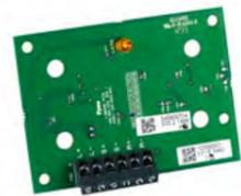
The FC410LI Line Isolator Module is designed to be used on the FireClass addressable controller loop. It monitors the line condition and when detecting a short circuit will isolate the affected section whilst allowing the rest of the loop to function normally. The purpose of the FC410LI Line Isolator Module is to ensure that, on a looped addressable system, no short circuit fault can disable more detection devices than would be lost on a conventional non-addressable fire circuit.
