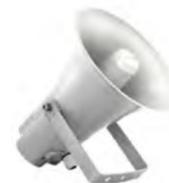
PS-30TN is a high performance voice alarm horn loudspeaker certified according to EN54-24 standards. Its broad frequency range, low distortion, and high volume ensure the delivery of intelligible voice and high quality sound. It is made of ABS and, for increased fire protection, the loudspeaker is equipped with built in ceramic connector blocks and a thermal fuse. The power taps are 15W/10W/5W @100V or low impedance 8 Ohms.
