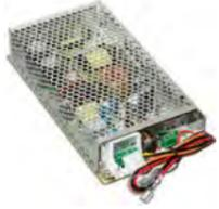
The BAQ is a power supply unit and battery charger to use with appliances that require a regulated voltage of 27,6 V and a maximum current of 5,5 A. Its power output is protected against overload, short-circuit and accidental inversion of the battery polarity.
