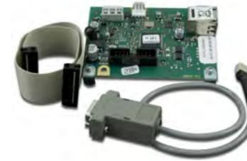
The FC500IP v3 is an IP Module which is used to connect control units in the FireClass 500 range to a LAN. With a public IP address, it is also possible to manage and monitor the control unit from anywhere in the world, as long as you have access to the Internet. The new version 3 is able to communicate events up to 3 receivers using SIA protocol.
