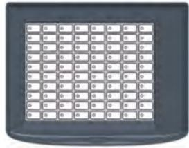
The FCZ8DS is a zonal LED display for FC600/FC700 systems. For every zone an alarm can be displayed by a red LED. The FCZ8DS contains 80 LEDs that can be assigned to any of the zones of the panel. Up to 3 FCZ8DS can be connected to a fire detection and alarm panel so that the status of all 240 software zones of the panel can be displayed.
