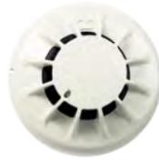
The 701P smoke detector operates by sensing the optical scatter from smoke particles generated in a fire. The micro-processor inside the detector allows for threshold compensation, meaning the detector will adjust sensitivity levels to compensate for dust and dirt levels in the chamber, resulting in fewer unwanted alarms and an extended detector life.
