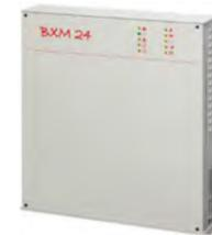
The BXM24/25-U and 50-U are approved by IMQ to EN 54-4:1997 + A1:2002 and EN60950-1:2001. The steel housing contains a 2.5 amp or 5 amp switch mode power supply and monitoring board and has space to accommodate 2 x 12V 17Ah sealed lead acid batteries. The 10 front panel LED's comprehensively indicate the status of the unit.
