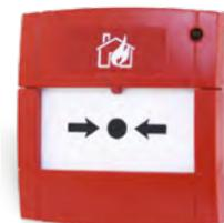
Conventional manual alarm call point with integral alarm LED and activation resistor. Operation is by break glass. This call point is semi flush mounted or can be surface mounted using back box 515.001.021 or 10-115, and comes with a test key.
