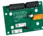
The FC410RIM Relay Interface Module provides one volt-free relay changeover contact on a latching relay. The relay is controlled by a command sent from the FireClass fire controller via the addressable loop.
