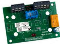
The FC410SIO Single Input/Output Module is designed to provide a monitored open collector input and a volt free relay changeover output. FC410SIO can switch up to 2 A @ 24 VDC.
