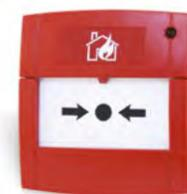
FC420CP-I Addressable Indoor Callpoint is designed to monitor and signal the condition of a switch contact that is operated by activating the deformable plastic element. A short circuit isolator is embedded.
