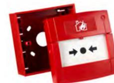
A conventional manual alarm call point with integral alarm LED and activation resistor. Operation is by resettable deformable element. Comes complete with a back box and a test key.
