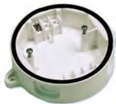
Where the detectors are mounted in humid and environmentally challenging situations such as marine or offshore installations, the 4B-DHM deck head mount provides a sealed waterproof mounting which protects the electrical connections in the base. Can be screwed, bolted / welded to the deck head. Supplied with 1 terminal. If more are required, use the optional base accessory.
