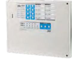
Designed and made according to EN54 standards, the J408 is a microprocessor based control panel for small to medium applications. It has 8 zones, each supports up to 32 detectors, for a maximum of 256 detectors. Each detection zone has an alarm-repeat output for selective management in the event of fire.
