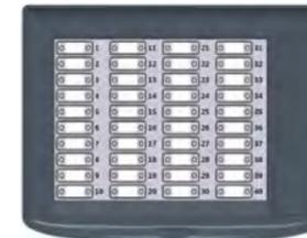
The FCZ4DS is a zonal LED display for FC600/FC700 systems. For every zone, an alarm or fault can be displayed by a red/yellow LED. The LEDs can be assigned to any of the zones of the panel. Up to 3 FCZ4DS can be connected to a fire detection and alarm panel.
