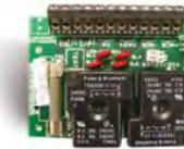
The SB520 sounder booster module enables the FC410SNM to drive circuits with higher currents whilst maintaining the reverse polarity integrity line monitoring. It is non-addressable and requires a local 24 V DC supply to drive a single circuit of polarized and suppressed sounders.
