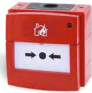
A weatherproof manual alarm call point with integral alarm LED and activation resistor making it compatible with the Prescient III Suppression Panel. Operation is by break glass. This call point is surface mounted and comes complete with back box and test key.
