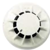
701H rate-of-rise heat detector detects abnormally high rates of rising temperature. The micro-processor inside the detector offers advanced algorithms resulting in improved false-alarm rejection rates. Can be used in areas where smoke detectors are unsuitable due to environmental conditions such as kitchens, locker rooms and canteens.
