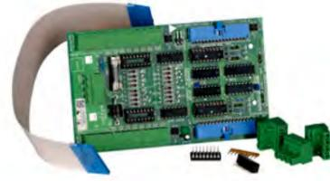
The XIOM is a 16 way universal input/output expansion board. The I/O on the XIOM can be set in banks of 8 to operate as follows:
