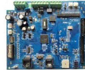
The MPM801 NexGen Multi-Purpose Interface Module is used to interface between the controller and the expansion modules through the Remote Bus. The MPM801 module is compatible with the legacy MPM800 module, except that the MPM801 module does not include the LCD or the keyboard interface. The MPM801 module provides remote connection over the new X-Bus for zonal displays such as the FCZ4DS, and FCZ8DS. The X-Bus also supports the ANN820, ANN840, and the ANN880.
