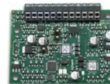
The FC410DDM provides the ability to connect and interface 2 conventional zones, to the FireClass fire alarm controller.
