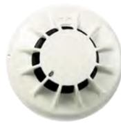
The 701PH optical heat detector operates by sensing the optical scatter from smoke particles generated in a fire, and a rapid rate of rising temperature increases the smoke detection sensitivity for normal ambient conditions, the high performance optical detector behaves as a normal optical detector.
