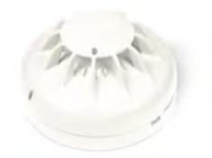
The FC400CH is designed to transmit digital signals representing the status of the carbon monoxide and heat elements of the detector. For use with the FireClass 500 panel.
