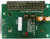
The FC410BDM Beam Detector Interface Module is designed to power and interface one FIRERAY 50/100/3000/5000 Beam Detector to the FireClass Digital Addressable Loop.
