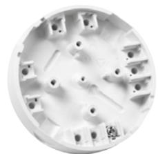
The euro-mounting base provides a matching back box, which allows the 5" bases to be ceiling mounted with conduit entries for standard 18 and 21mm conduit.
