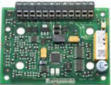
When activated, either by a fire signal or by a fault or isolation within the fire door zone, the FC410TSM will interrupt the supply to the door holders and the doors under control of the module will close. The module has the provision to monitor a contact to report to the fire controller if the door fails to close. The module also includes a built-in line isolator.
