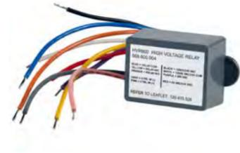
The HVR800 High Voltage Relay Interface is a non-addressable multi-voltage relay module (operating from 24V DC, 24V AC, 120V AC and 240V AC). The encapsulated HVR800 provides a 10 amp volt-free contact that can be used to extend the contact ratings of FC410RIM Addressable Relay Module applications.
