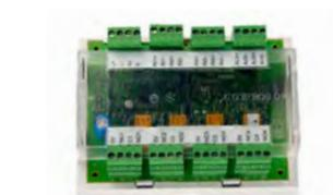
The FC410QIO Quad Input/Output Module is designed to provide four monitored digital inputs and four potential free relay changeover outputs. The outputs can be connected to an Auxiliary Voltage source and its voltage can be monitored.
