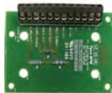
In many cases it will be necessary to site the FC410BDM Beam Detector Module some distance from the beam detector itself. To minimize and simplify wiring in such cases an optional unit, the BTM800 beam termination module is available.
