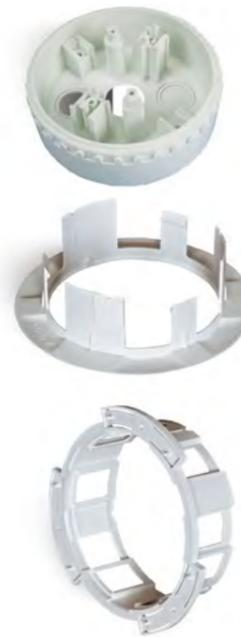
The Time Saver Ceiling Tile Adaptor is used with the 4B 4" detector base snap fit base and consists of three parts, a bezel and clamp that are fitted to the ceiling tile and a back-box that carries the detector and base assembly.
