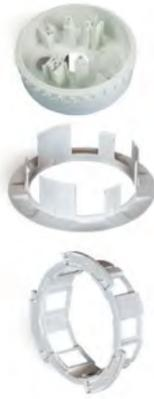
The time saver ceiling tile adaptor is used with the 4B 4" detector base snap fit base and consists of three parts, a bezel and clamp that are fitted to the ceiling tile and a back-box that carries the detector and base assembly. Requires a 127mm diameter hole. The CTA adaptor plate allows this to be used with other devices such as the FC430SB.
