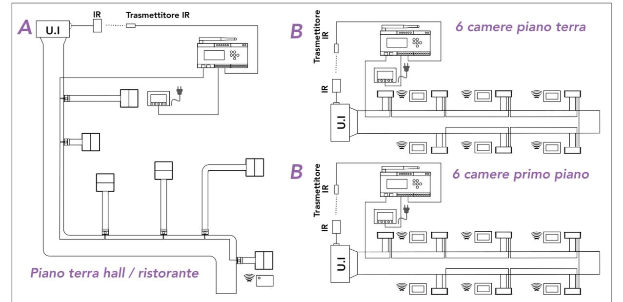
✓ **INSTALLARE LA CENTRALINA IN UN VANO TECNICO O NEL QUADRO ELETTRICO**
