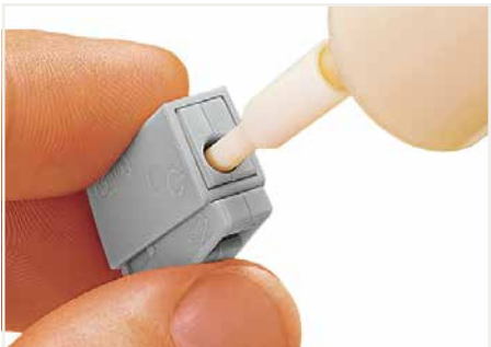
WAGO Lighting Connectors Push nozzle of the “Alu-Plus” syringe first into the circular and then into the square conductor entry hole of the WAGO lighting connector.
