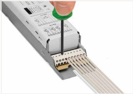
Removing a conductor via 1.0 mm Ø 206-841 Disconnection Tool.
