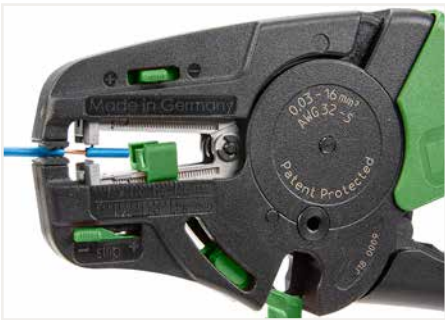
Partially stripping a conductor.
