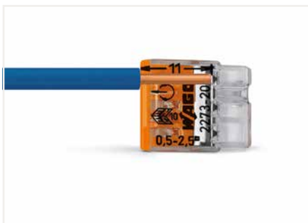
Strip solid conductor to 11 mm/0.43 inch (see marking).
